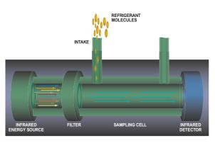
The filtered infrared energy passes through the sampling cell, striking the infrared detector. D-TEK Select is ready to sense any refrigerant.
